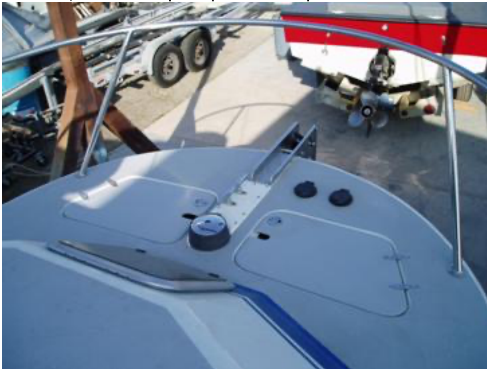
Here is the Maxwell Freedom 800 windlass and foot switches and heavy duty Bruce type bow roller. The dual anchor lockers come standard on our boats.
