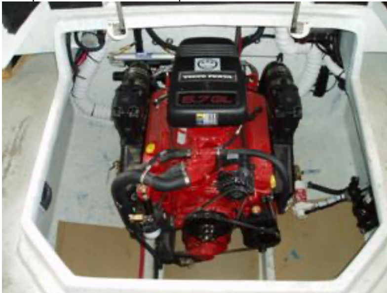
Bob's boat is powered by a Volvo 5.7 ltr gas engine. His mechanic will thank him when he brings the boat in for service because Bob's bait pump and filter on his salt water wash down as well as everything else in the engine compartment are easy to get to. There is a nice raised combing on the front and sides and a deep trough across the back to keep the water out.
