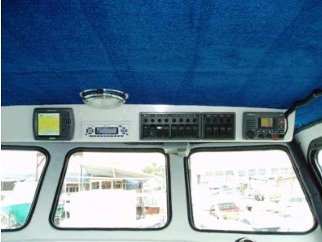
Overhead electronics box with stereo, VHF, extra GPS and switch panel. The overhead light can be white or red
