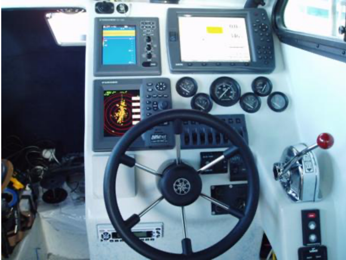
There is a separate GPS, radar and sounder. In addition, there is a cell phone power booster port.
