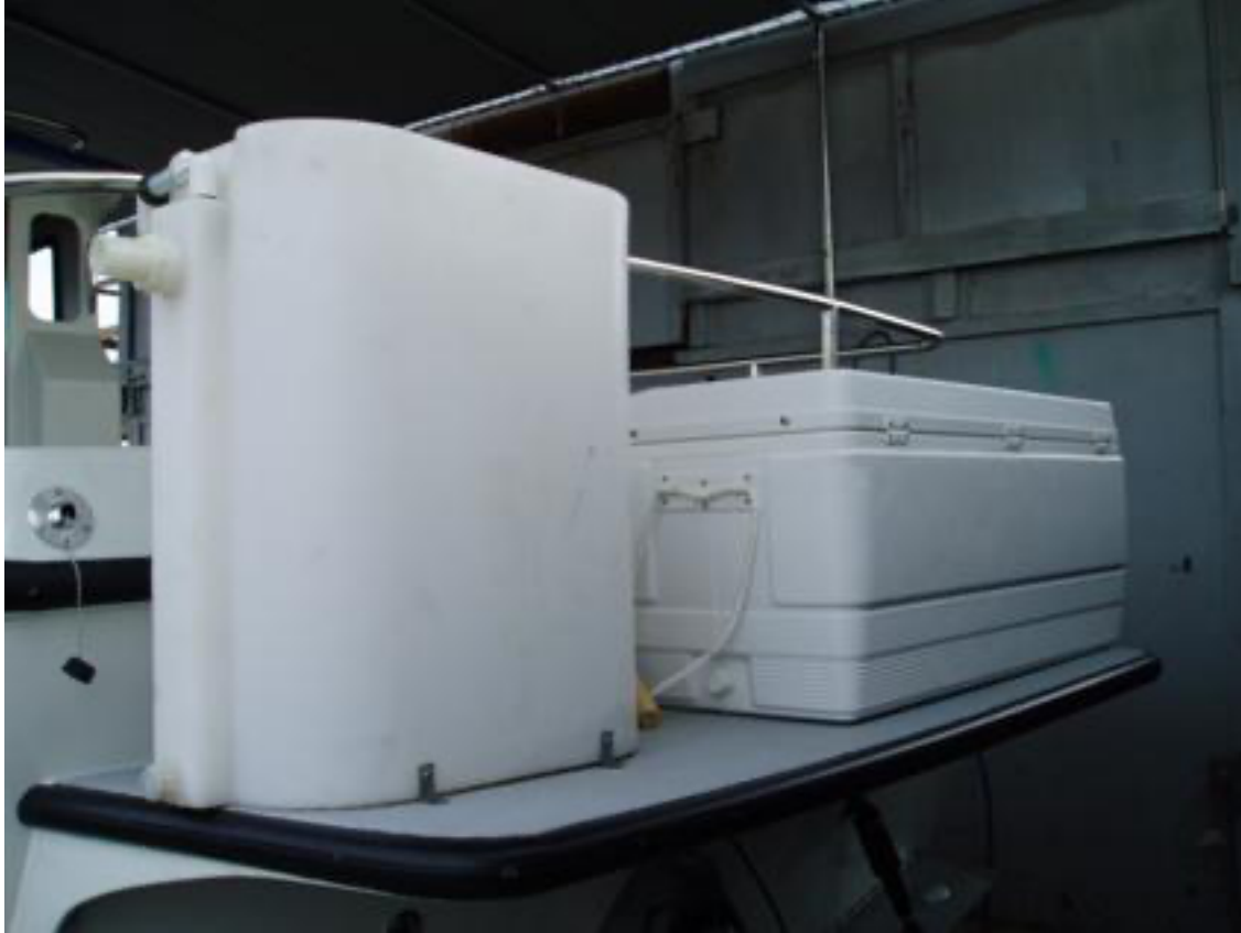
Bob's bait tank and ice chest on the swim step. The dive ladder pulls out from under the swim step and the bait tank and ice chest are removable
