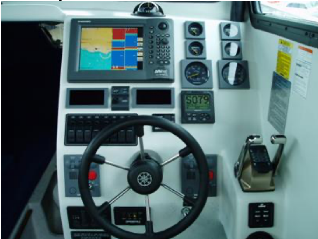
Shown above: Paul's Furuno NavNet has a big screen and gives you GPS, sounder and radar
