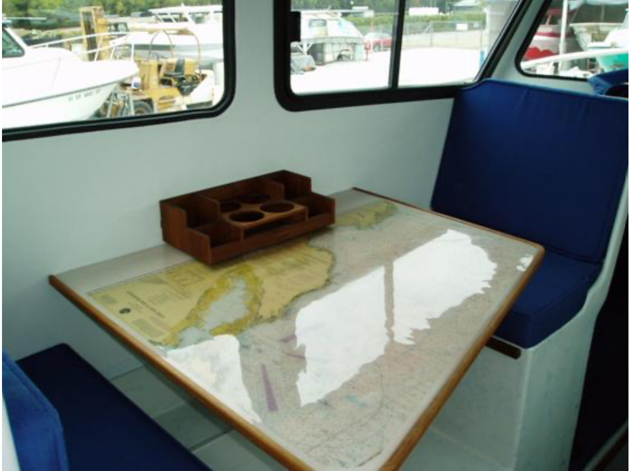
Here is Paul's custom dinette table with a chart of the area he fishes in Northern California. The table moves down to become an extra bunk
