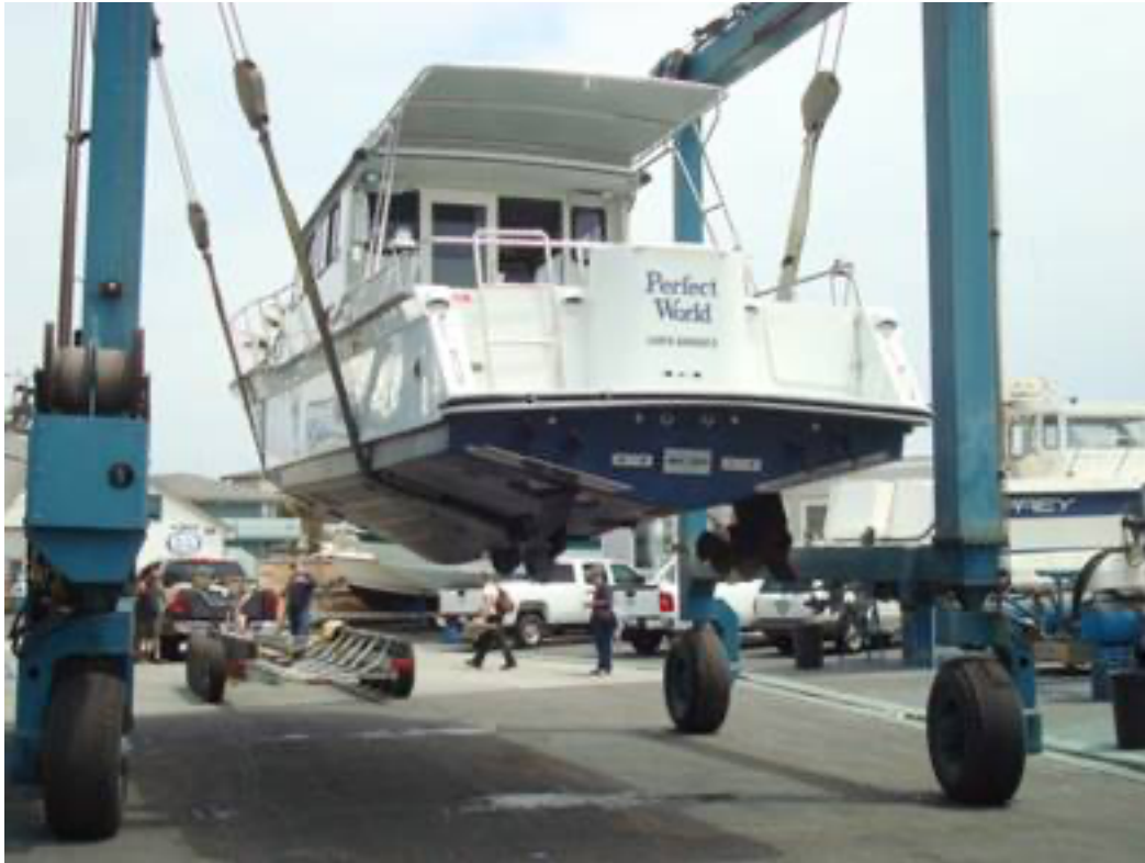
Damon from Harbor Marineworks prepares for the splash - you can see the Volvo IPS drives on the bottom of the hull
