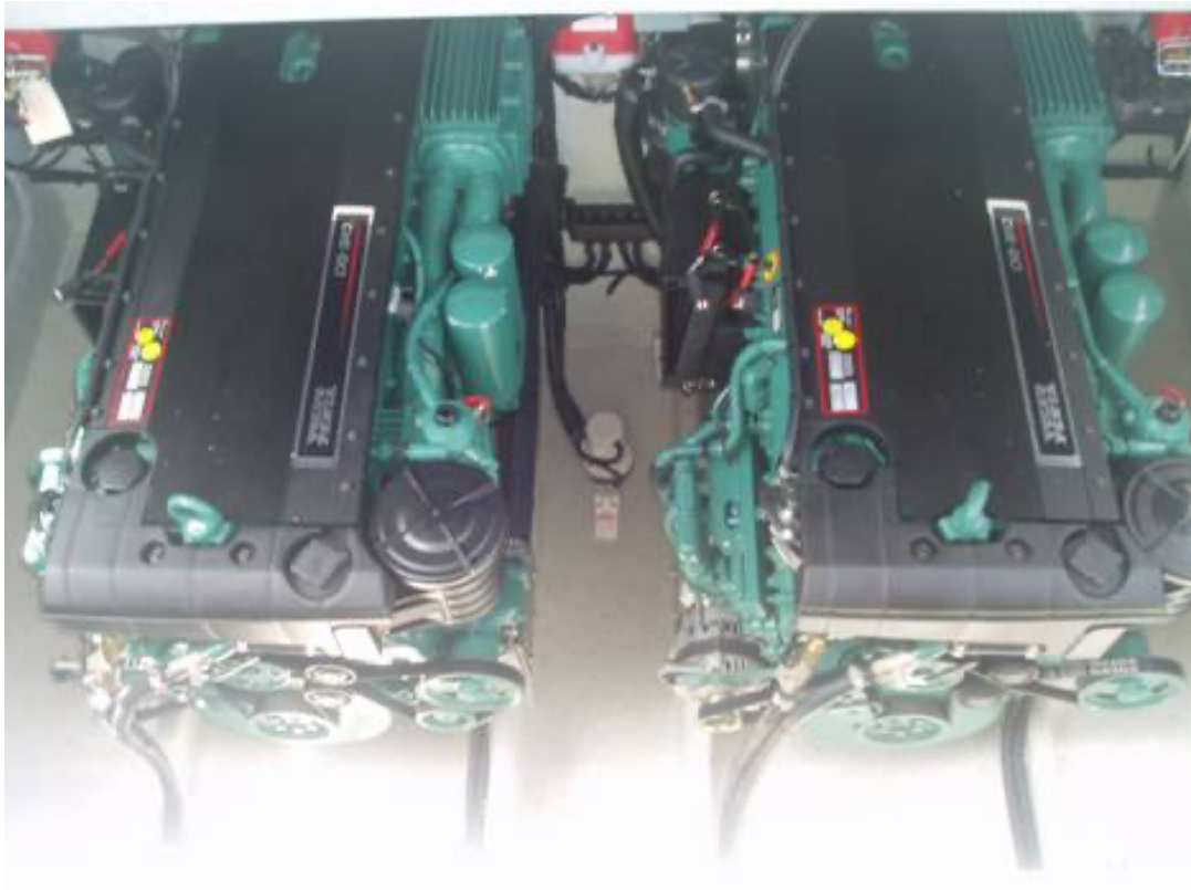
Twin 310 HP Volvo D6's power the 33'
