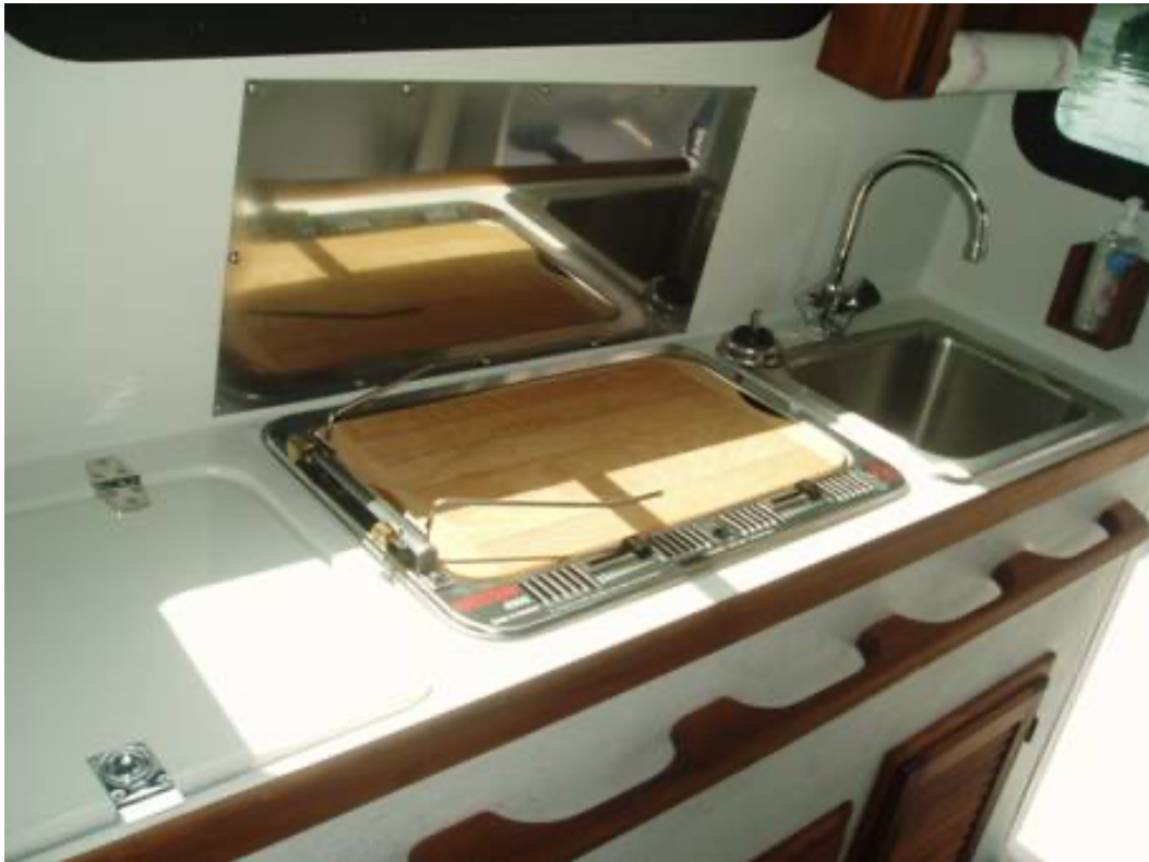
The galley with built-in fridge in counter to the left
