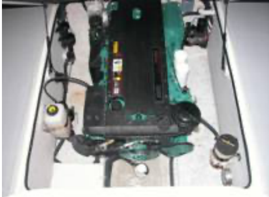
Volvo D6 350 HP diesel engine - this engine compartment showcases how important it is to have easy access while working on the engine
