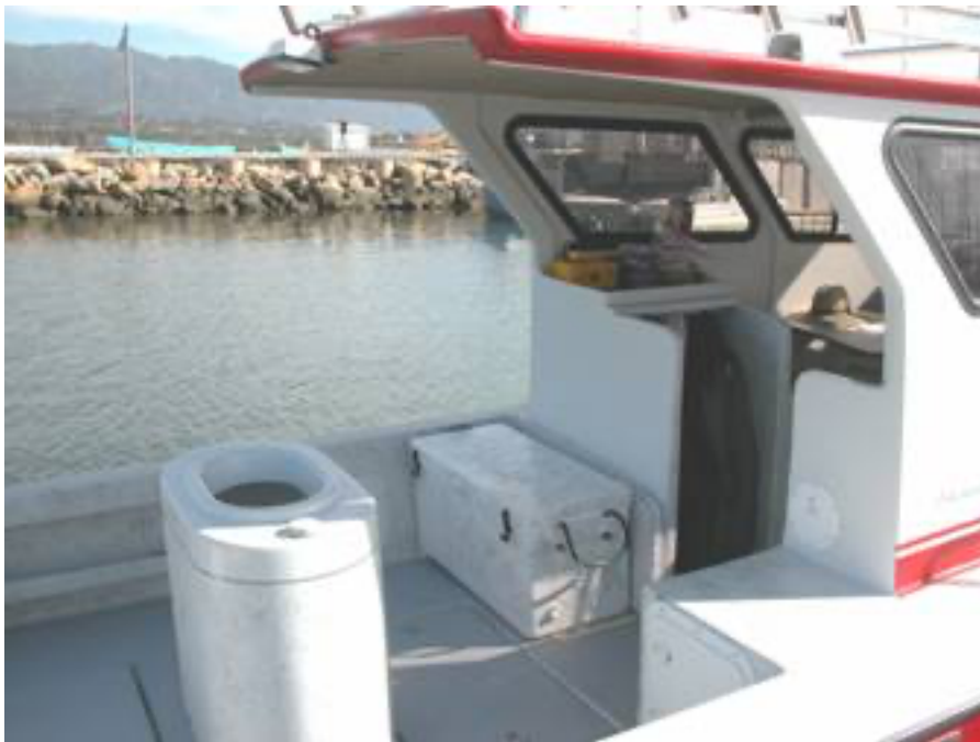
The extended overhead gives added shade. Also shown here is the aft step down head, fiberglass bait tank and removable ice chest.
