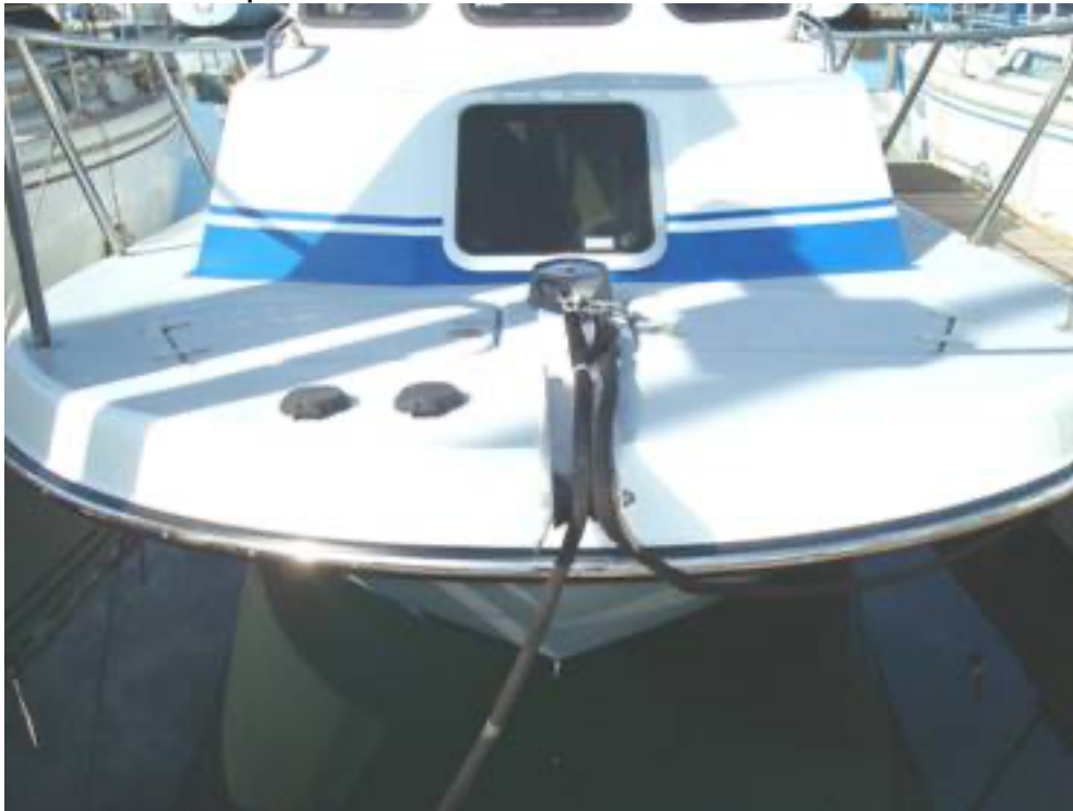
Two anchor lockers and Maxwell windlass
