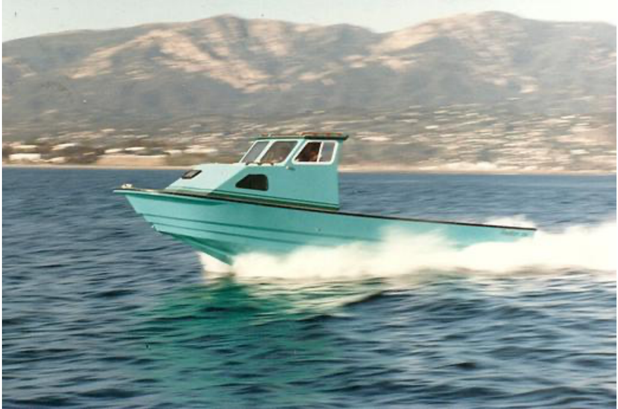
1985 26 x 8'6" with 250 HP diesel engine and V-drive
