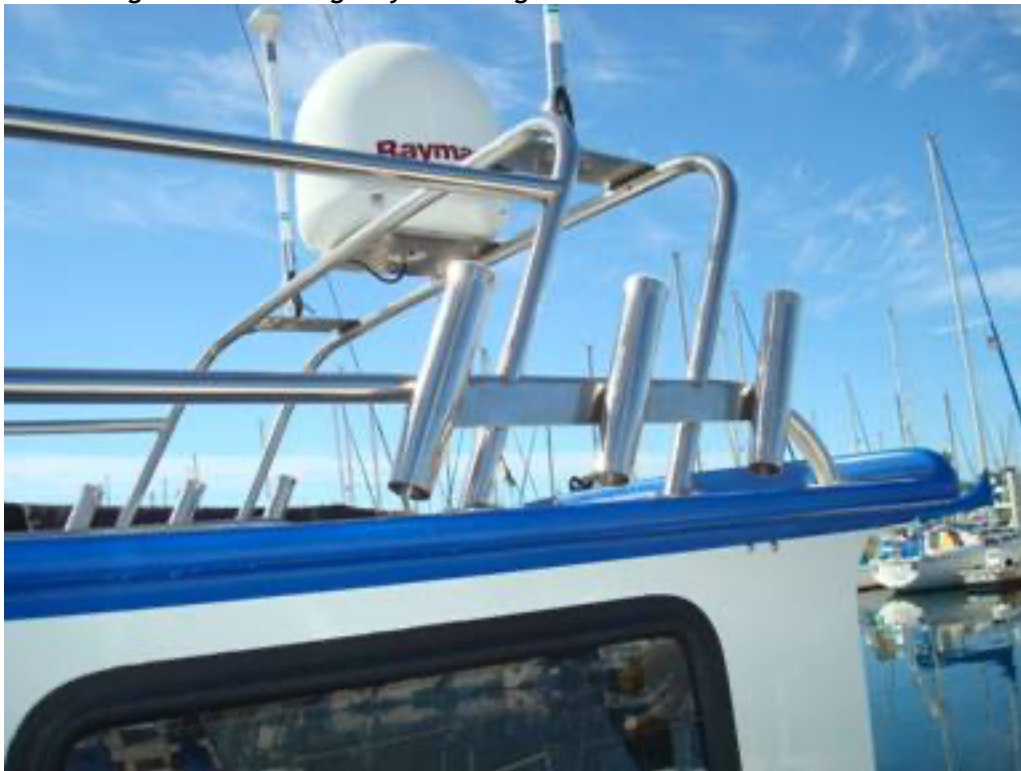
Stainless surfboard/kayak racks and stainless rocket launchers
