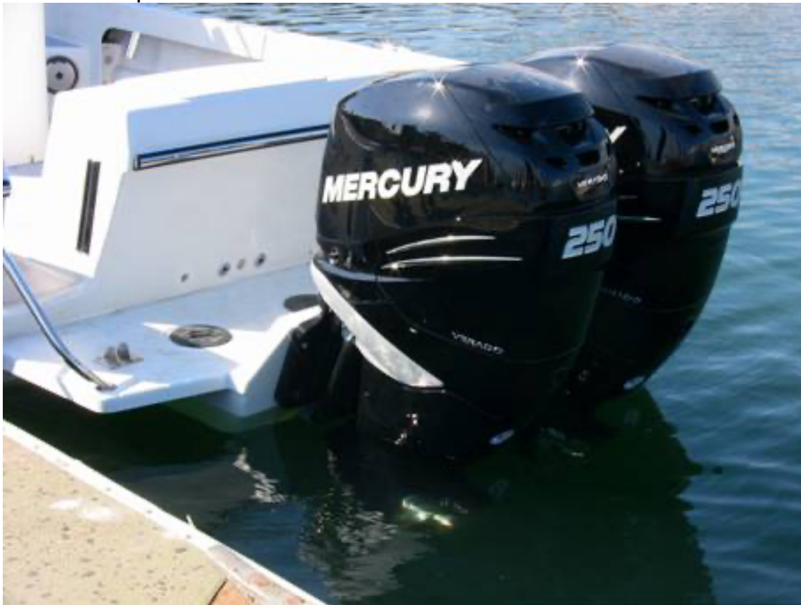
Twin Mercury 250 HP Verados mounted on a Hermco fiberglass flotation swimstep bracket
