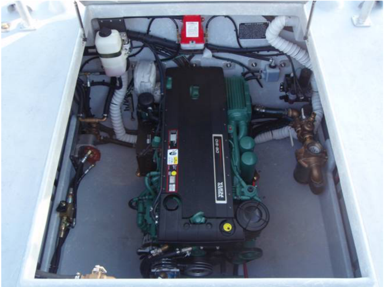
The boat has a Volvo D-6, 310 HP diesel engine
