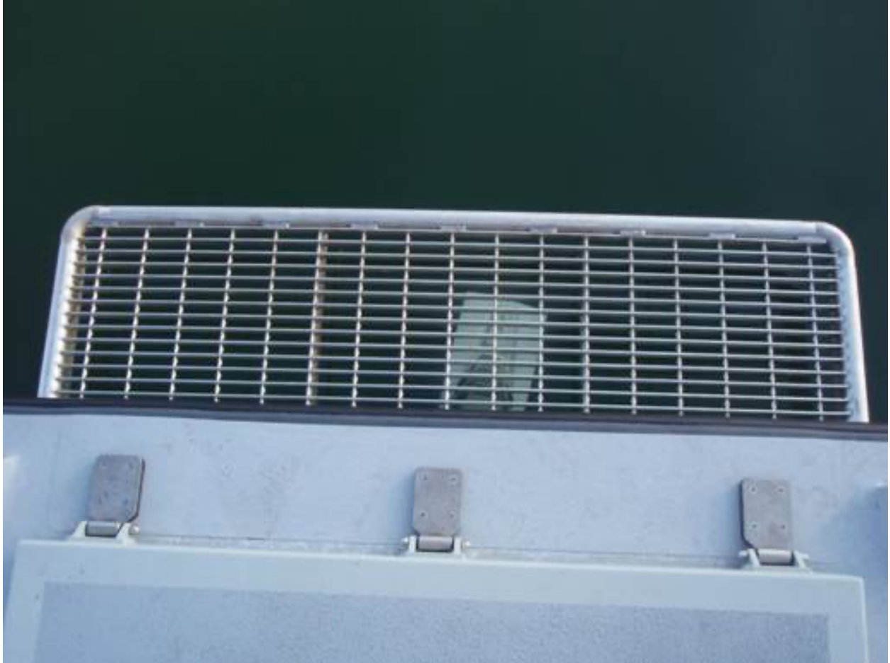
The swim step, as well as the hatches and stern rail, were built out of aluminum by Hendrix Manufacturing in Goleta
