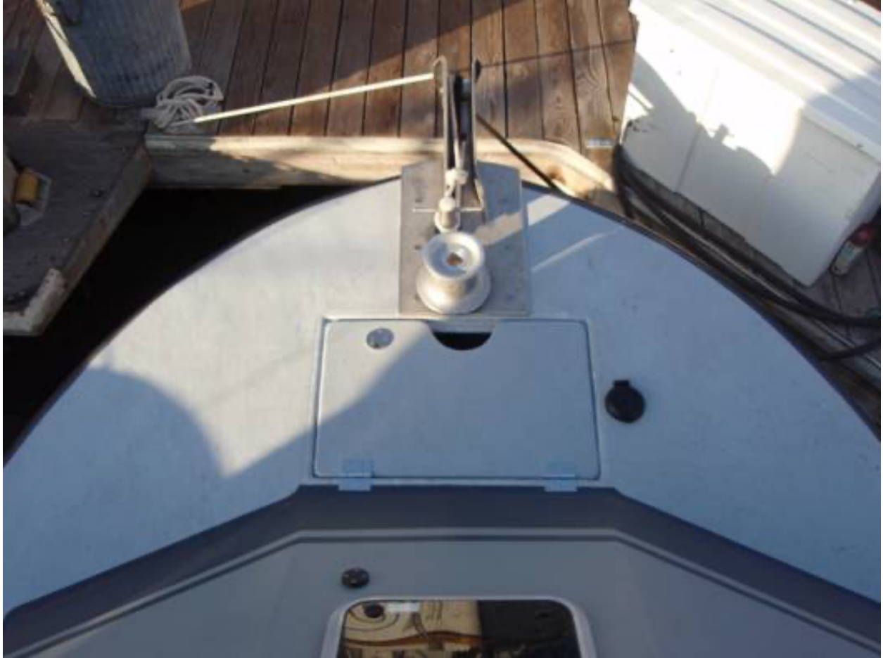
This shows the anchor puller and a custom bow roller, also built by Hendrix
