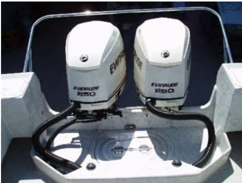
The Kauai boat is powered with twin Evinrude ETEC 250 HP outboards. There is a stainless steel rope guard surrounding the outboards.
