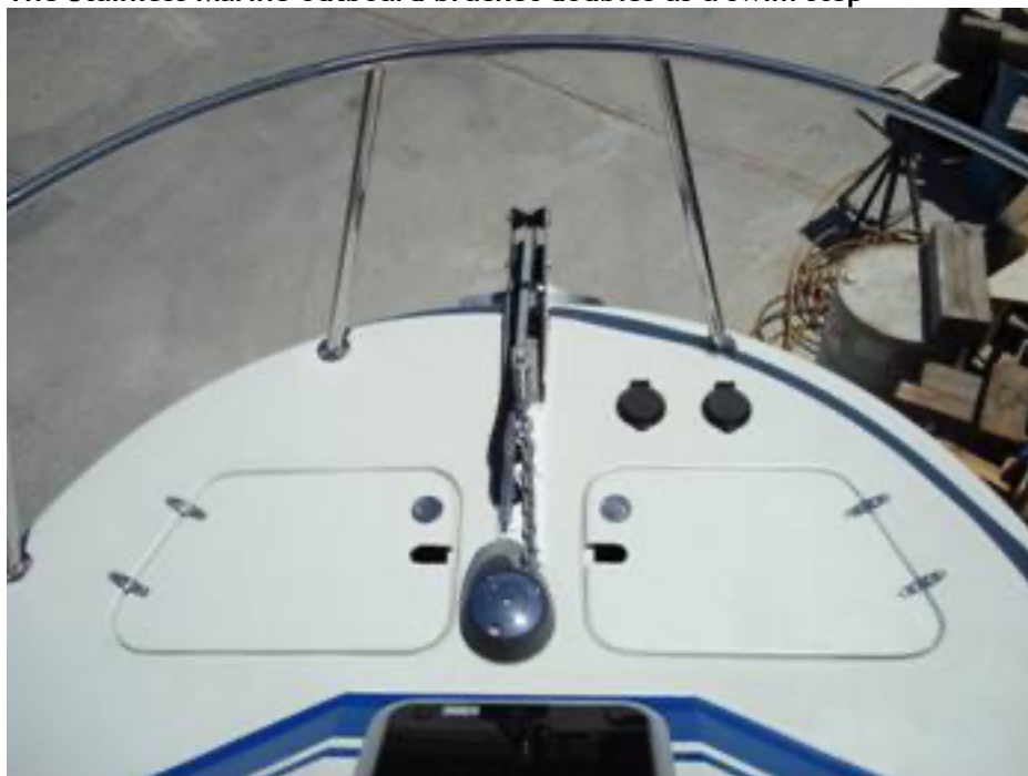
The bow with the Freedom 800 windlass and dual anchor lockers
