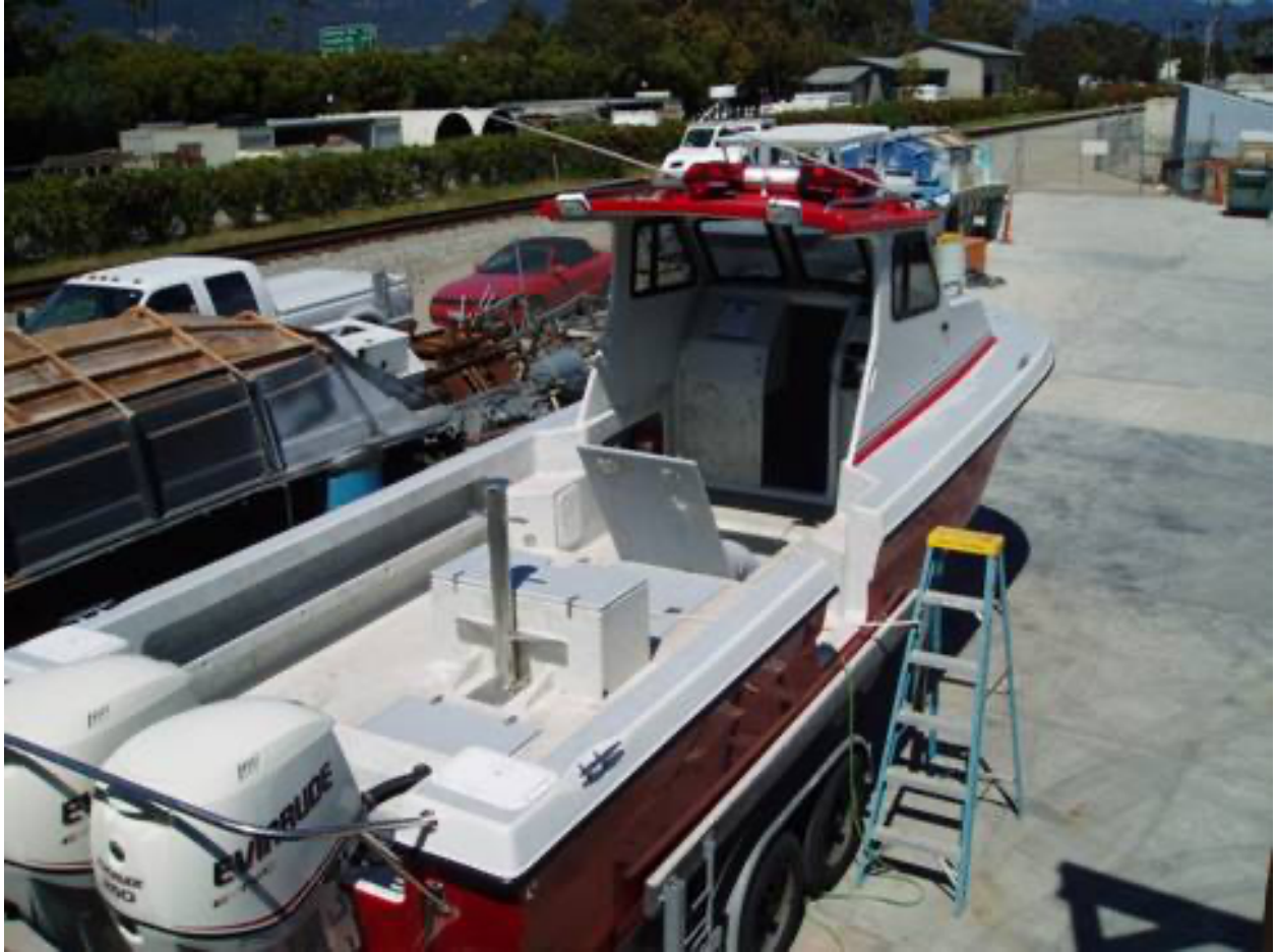
Here is the deck layout with the tow bit and rope locker in mid deck
