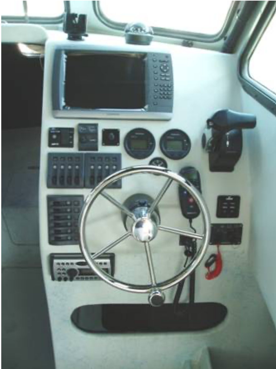
Tony has the new Garmin 4212 Network chart plotter, in the upper left of the dash. His Garmin system includes chart plotter, GPS antenna, satellite weather module, Digital remote sonar, transducer and temperature probe.
