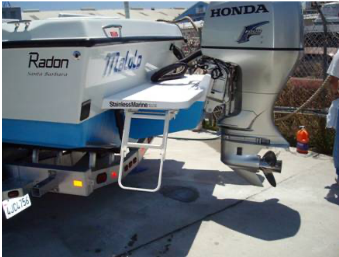
The Stainless Marine outboard bracket doubles as a swim step
