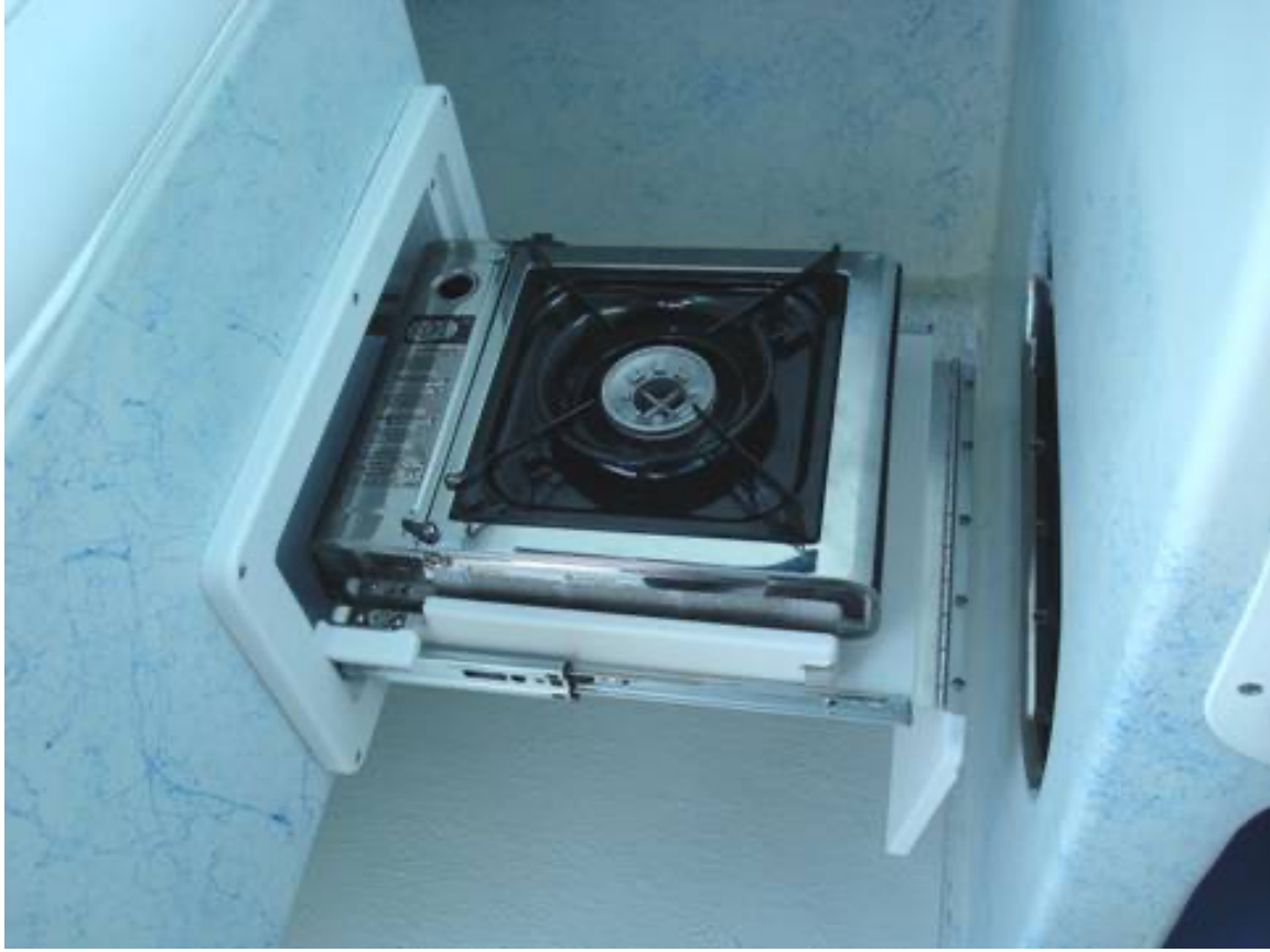
This is a pull-out drawer with a stove top inside...
