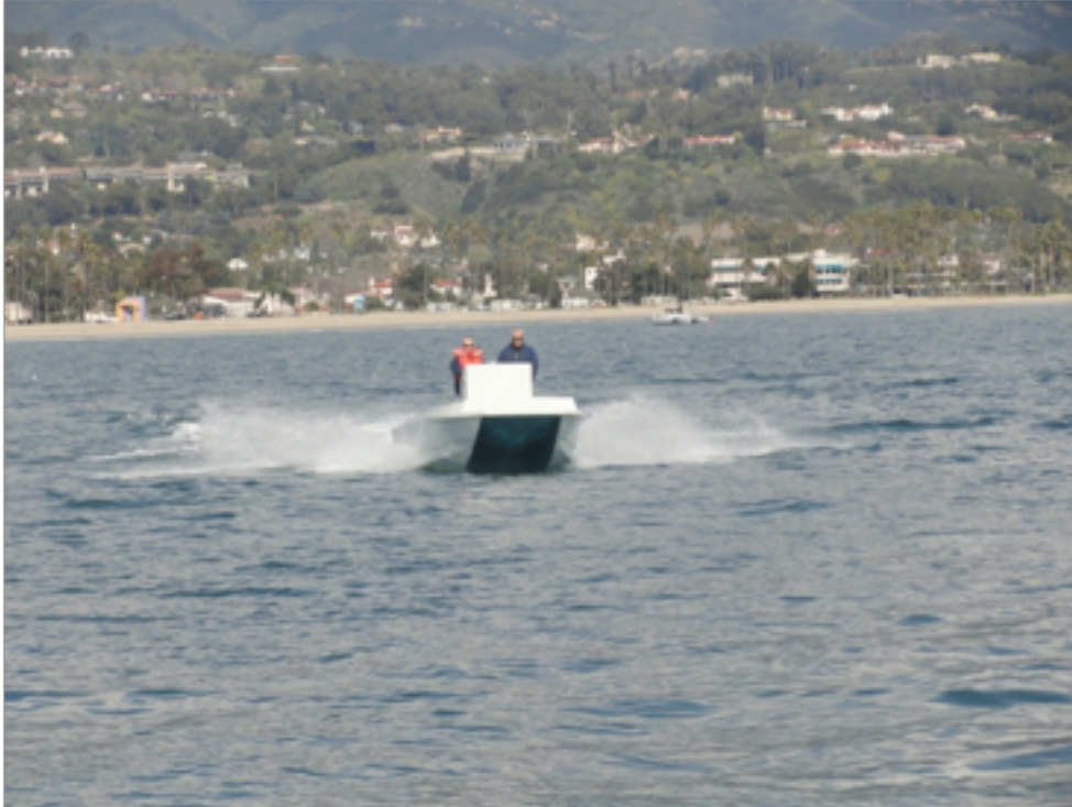
Don and Mike Armstrong get the prototype “Radamaran” out for a sea trial. The design is based on the “catamaran” design, coupled with the “Radon” hull
